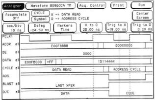
Timing waveforms can be displayed with data values and symbolic information to illustrate bus cycles and data flow.
